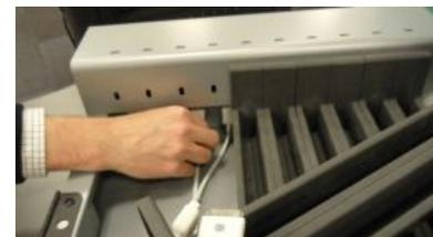
5. Plug the USB end of the replacement cable into the appropriate USB port on the right side of the open pocket.
