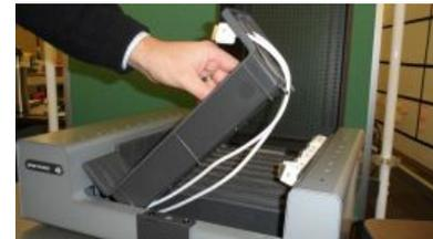
4. Unplug the cable from the USB ports, and pull the USB end through the holes in the pocket.
