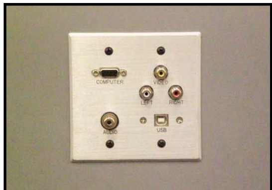
STEP 3B: Using the four 6-32 x 1/2" flat head screws provided with the plate and the four 6-32 hex nuts (DD), install the data pass through plate to the side panel.
