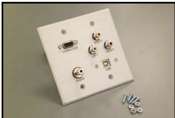
STEP 3B: Using the four 6-32 x 1/2" flat head screws provided with the plate and the four 6-32 hex nuts (DD), install the data pass through plate to the side panel.
